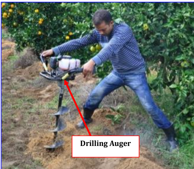
Use of drilling auger to prepare the pits (holes) for the installation of the buried diffusers for orange trees in Beni Khaled, Cap Bon North of
