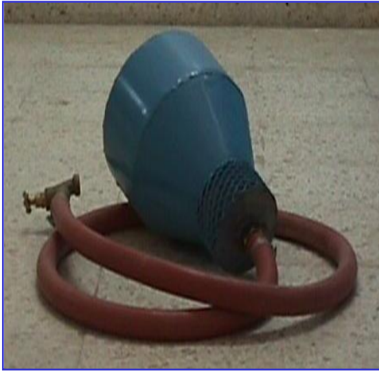
Small sized draining floater for small water rain water storage concrete reservoirs
