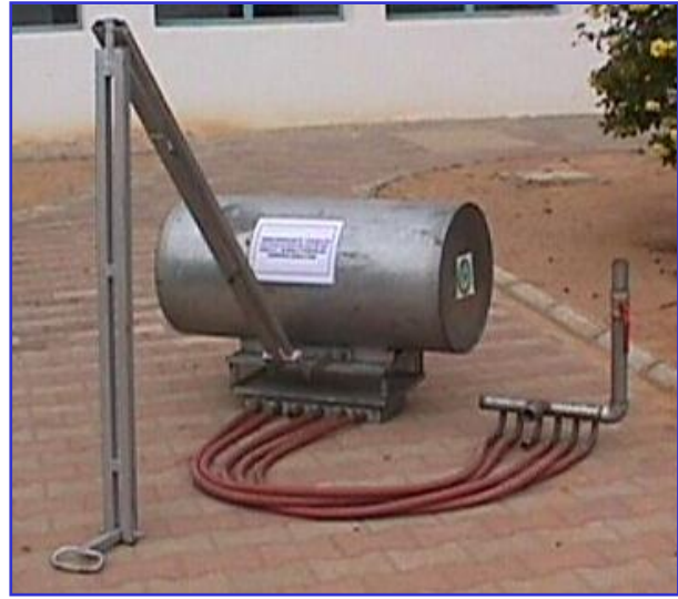
Middle sized draining floater for middle dams (1000 till 10000 cubic meters)
